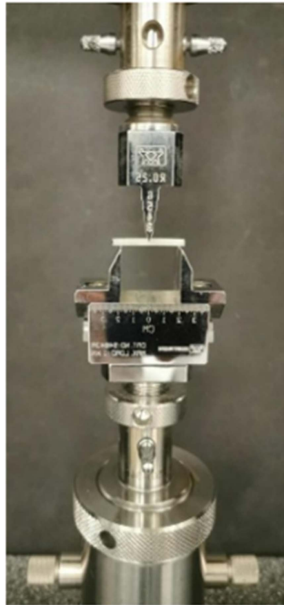
Figure 2. Sample placed in universal testing machine (Instron) and subjected to a three-point bending test.
